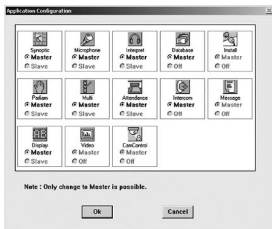
The Multi PC software module is needed when more than one PC is required to control the DCN Next Generation system. All Slave PCs in a multi-PC environment are connected via Ethernet to the Master PC, which is connected to the CCU.
