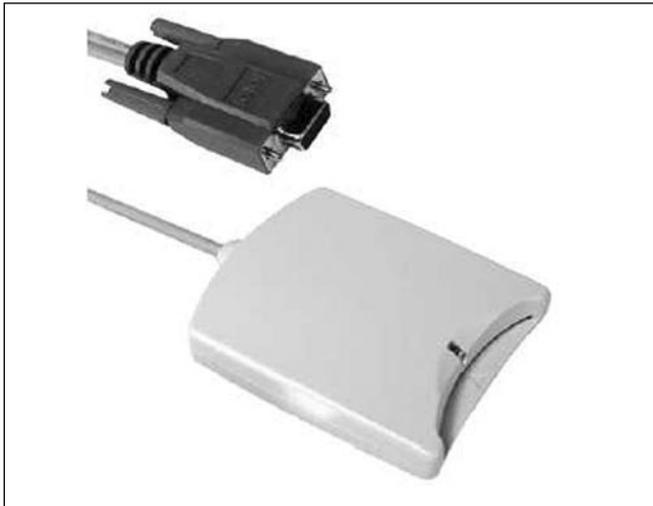
Used in combination with the ID Card Encoder software module (LBB 4181/00), the LBB 4157/00 encodes delegate ID cards (LBB 4159/00).
