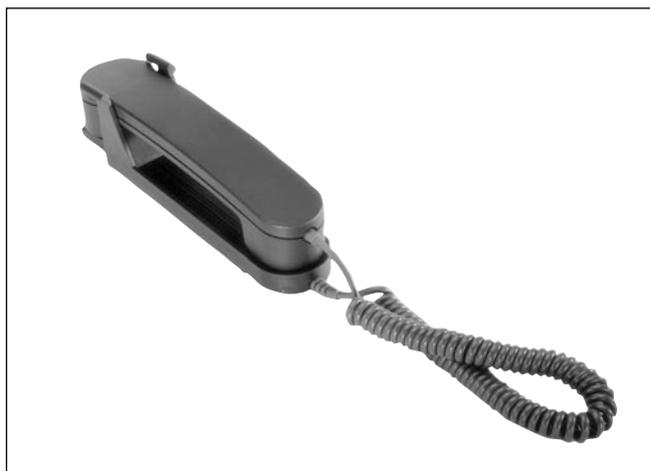
Lightweight and compact, this robust and attractively styled handset and cradle enables private 2-way conversation between conference participants. The handset is hard-wired to the cradle by a coiled cable, 0.5 m (19.6 in) long when coiled, and 2 m (78.7 in) uncoiled. The cable is terminated with a six-pole RJ45 connector for connection to Concentus and Dual Delegate Interface. When used in permanent installations, the unit is easily mounted to a tabletop or wall using the two screws.
