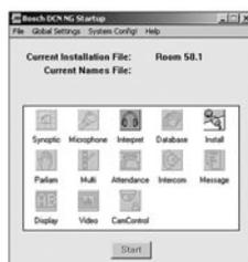
The Startup screen is active whenever DCN Next Generation software modules are used for controlling and monitoring. This module is different from other DCN Next Generation software modules as it is primarily used as a platform from which the other modules are selected. However, this is only one aspect of Startup. The following can also be carried out:
