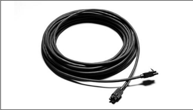
This is a special cable with 2 plastic fibers for data and audio communication and 2 copper cores for the power supply. The cable is supplied with the network connectors fitted. This cable can be used to connect the CCU to audio expanders.
