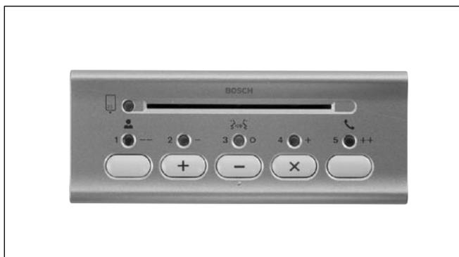
The Voting and Card Panel has the same functionality as the voting panel DCN-FV and extended with an ID card reader. The ID card reader enables identification of delegates to the DCN Next Generation system as well as providing a convenient facility that ensures only authorized delegates can participate in voting sessions or general conference proceedings such as microphone use.
